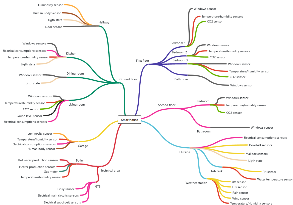
Figure 2: Sensors deployed in the smart house
