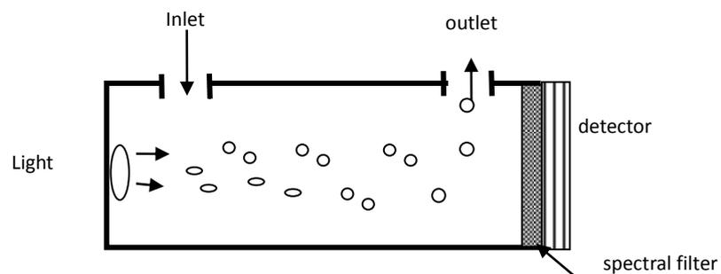
Basic mathematical model: A majority of both organic and inorganic polyatomic gases have specific absorptive wavelengths in the infrared region. When infrared light passes through, the light transmissivity of this gas molecule at a certain wavelength can be expressed by Lambert-Beer Law:
